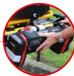
Fig 3 Patient box released from corpuls3 bracket. Patient box can quickly mount and de-mount to/from the stretcher.
