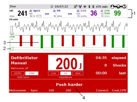
Fig. 5-21 CPR feedback
