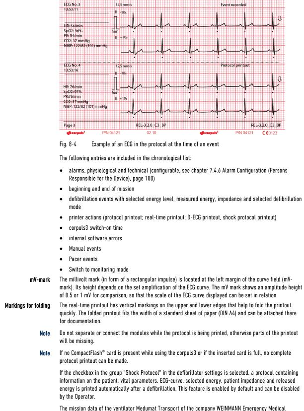
The mission data of the ventilator Medumat Transport of the company WEINMANN Emergency Medical Technology GmbH + Co. KG can be printed out on the corpuls3 by means of the Bluetooth® interface.
