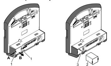
Fig. 10-3 Changing the battery (monitoring unit)
