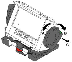
Fig. 5-2 Removing the shock paddles from their holders
