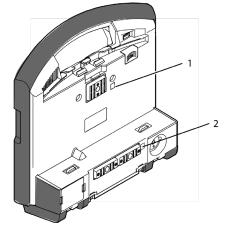
Fig. 10-4 Monitoring unit, infrared interfaces
