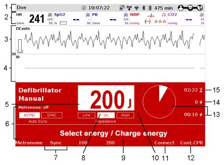
Fig. 5-8 Manual defibrillation, initial screen (illustration may differ)
