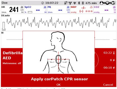
Fig. 5-20 CPR feedback, attaching the corPatch CPR sensor
