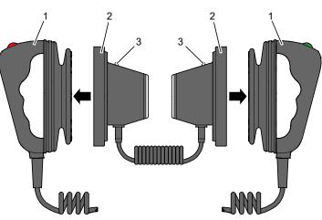
Fig. 5-11 Connecting baby shock electrodes
