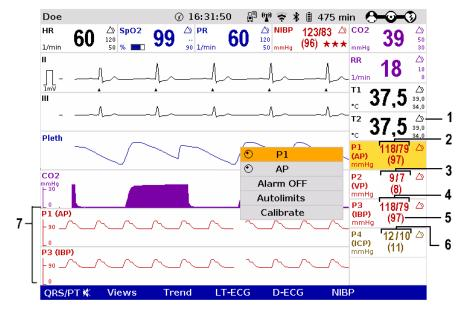
Fig. 6-37 IBP monitoring, configured screen
