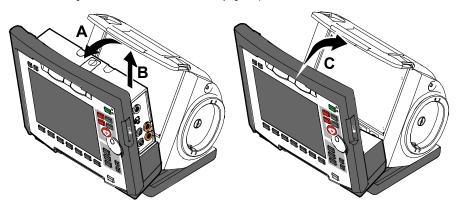
Fig. 4-25 Removing the patient box from the compact device (illustration may differ)
