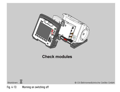
In this case, separate the modules and check whether all modules have been shut down. If this is not the case, switch off the modules which have not been switched off by pressing the respective **On/Off** key.
