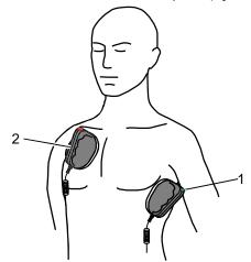
Fig. 5-10 Applying the shock paddles
