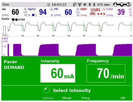
Fig. 5-16 Pacer, selecting the intensity
