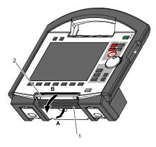
Fig. 10-1 Opening the printer flap
