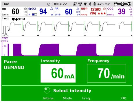
Fig. 5-13 Pacer pulse identification
