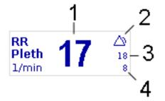
Fig. 6-24 Parameter field Respiration rate over pleth
