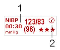
Fig. 6-35 NIBP parameter field with active interval measurement
