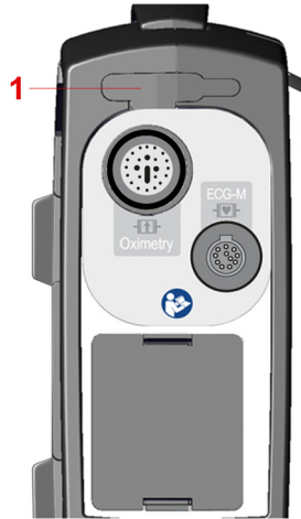
Fig. 6-5 Inserting SD card (pictured: right side of device without corPatch CPR)
