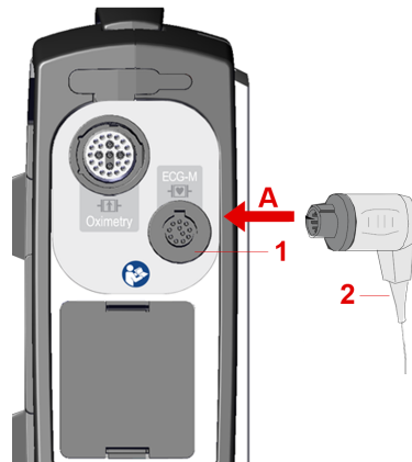
Fig. 10-3 Connecting ECG electrodes (example without corPatch CPR sensor)
