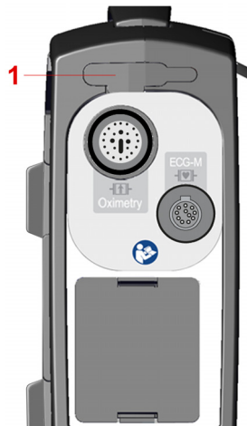
Fig. 6-6 Inserting SD card (pictured: right side of device without corPatch CPR)
