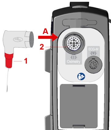
Fig. 10-5 Connecting a pulse oximetry sensor (pictured: right side of device without corPatch CPR)
