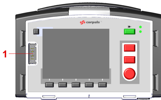
Fig. 5-1 Interfaces at the front side of the device (illustration without pacer option)
