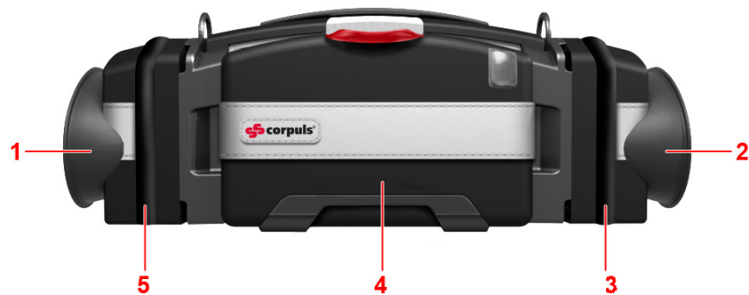
Figure 19-1 corpuls1 with accessory bags and front cover and shock paddle holders
