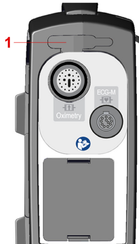
Figure 6-6 Removing SD card (pictured: right side of device without corPatch CPR)
