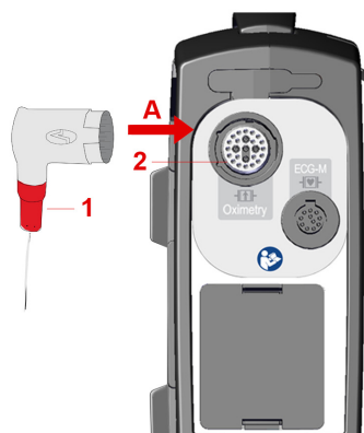
Figure 10-5 Connecting a pulse oximetry sensor (pictured: right side of device without corPatch CPR)
