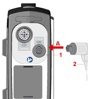
Figure 10-3 Connecting ECG electrodes (example without corPatch CPR sensor)
