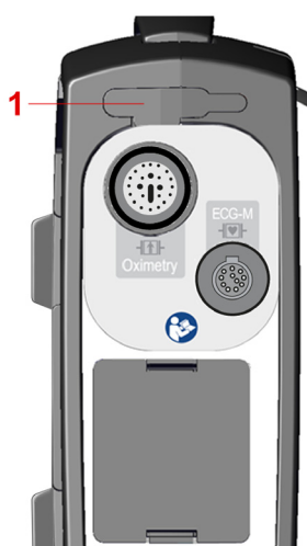
Figure 6-5 Inserting SD card (pictured: right side of device without corPatch CPR)
