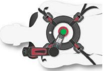
Close the locking lever by slapping it with the palm of your open hand and then press the green or amber LED start / stop button.
