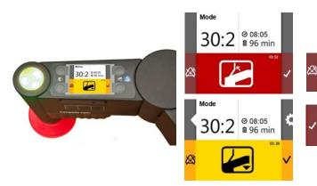
Activate and deactivate alarm suspension by pressing the soft key located beside the alarm symbol, for 3 seconds.
