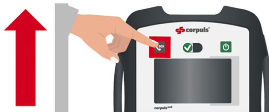
Fig. 6-2 Pictogram Press Emergency call button (fully automatic corpuls aed model with emergency call)
