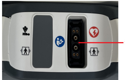
Fig. 6-4 Socket for corPatch easy therapy electrodes
