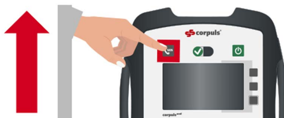
Fig. 5-3 Pictogram Press Emergency call button (Semi-automatic corpuls aed model with emergency call)
