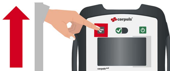
Fig. 5-2 Pictogram Press Emergency call button (fully automatic corpuls aed model with emergency call)
