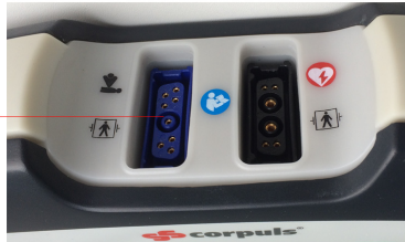
Fig. 6-14 Socket of corPatch CPR disposable sensor
