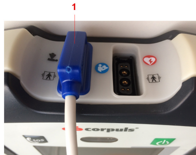
Fig. 6-15 Connected corPatch CPR disposable sensor
