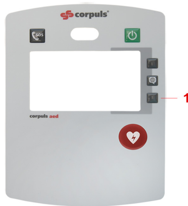
Fig. 6-11 Semi-automatic model with [Analyse] softkey
