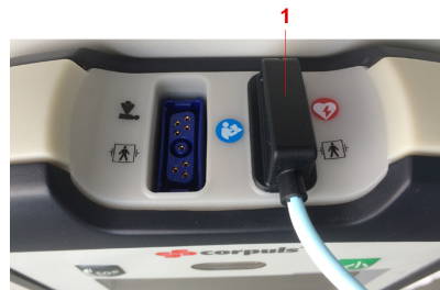
Fig. 6-5 Connected corPatch easy therapy electrodes
