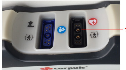
Fig. 6-4 Socket for corPatch easy therapy electrodes
