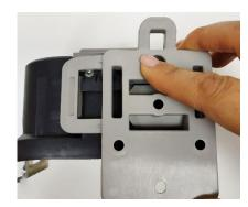
Figure 5: Locating the *Mount Adapter* on the Warrior lite Base Unit back side, then sliding it to the left
