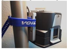
Figure 3: Warrior lite mounted to a Pole using a strap
