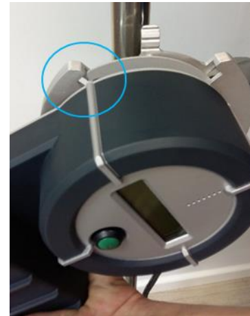
Figure 6: The Base Unit left hole is in front of the Left slit back
