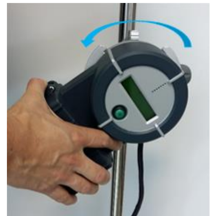
Figure 8: Sliding the Base Unit counterclockwise
