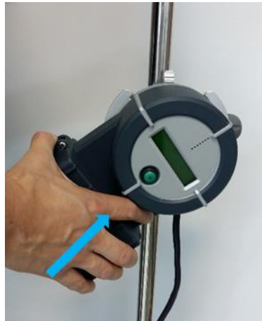
Figure 5: Inserting the Base Unit back wall to the Right slit of the QiF™ Pole Mounting Unit
