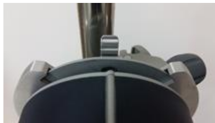
Figure 9: The Lock latch is inside the Base Unit back wall upper hole
