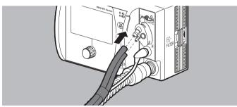
3. Connect the flexible oxygen tube and pressure measuring tube.
