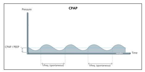
The CPAP / PEEP setting increases the lower pressure level during spontaneous breathing. This results in an increase in the functional residual capacity of spontaneously-breathing patients. The patient is able to breathe spontaneously without any restriction at the set pressure level. The CPAP mode is used exclusively on patients with adequate spontaneous breathing.
