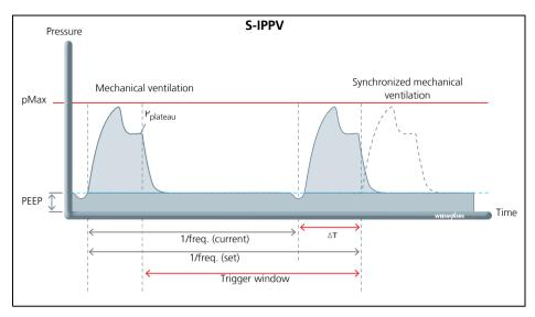
S-IPPV mode is used for volume-controlled ventilation at a variable mandatory minute volume. Throughout the entire expiratory phase, a trigger is active which enables the patient to trigger a new mechanical breath. This means the patient is able to increase his or her respiratory rate – and thus the minute volume – as needed. As a rule, this mode is used on patients who have inadequate spontaneous breathing.
