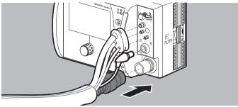
1. Connect the ventilation hose to the ventilation hose connection.
