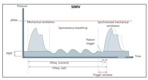
The SIMV mode is used for volume-controlled ventilation at a fixed mandatory minute volume. The patient can breathe spontaneously between the mandatory mechanical breaths and thereby increase the minute volume. During spontaneous breathing, the mandatory mechanical breath is synchronized with the patient's breathing. The mandatory minute volume and the mandatory respiratory rate remain unchanged. The set maximum pressure limit (pMax) ensures the safety of the patient.
