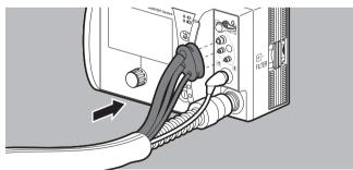
3. Attach the measuring circuit connector to the measuring circuit connection.
