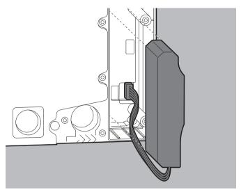
1. Attach the battery's electrical connector. To do so, plug the battery connector into the socket.
