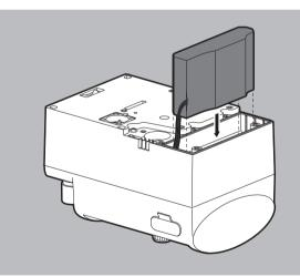
2. Insert the rechargeable battery. Pay attention to the cable routing when doing this.
