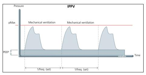
IPPV mode is used for mandatory, volume-controlled ventilation at a fixed tidal volume. This mode is used on patients who have no spontaneous breathing. However, a spontaneously breathing patient can breathe deeply and freely during expiration. The set maximum pressure limit (pMax) ensures the safety of the patient.
