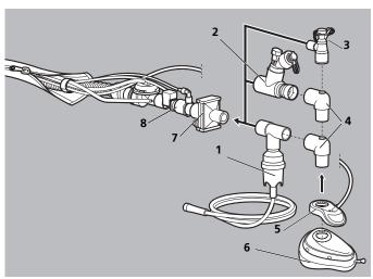
Place the mask/tube 6 (optionally with elbow 4 and/or MEDUtrigger 5) on the nebulizer 1, 2 or 3.
