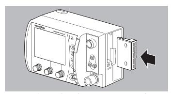
2. With the filter side facing forwards, slide the hygiene filter into the device's filter compartment until the hygiene filter is flush with the device.
