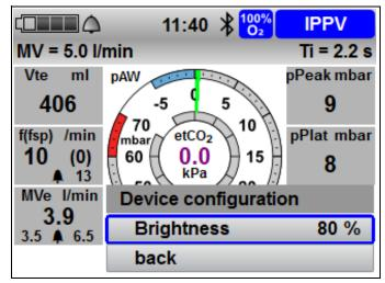
Here you can change the brightness of the screen. Settings between 5 and 100% are possible. The selected setting is retained after switching off and on again.
