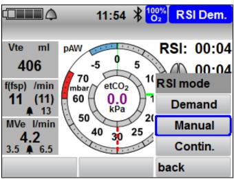
2. To select the **Manual** function, switch to the **Manual** field using the right-hand navigation knob.
