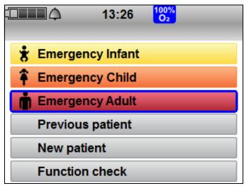
If the device was switched off for < 30 seconds (e.g., for a battery change), a countdown in the **Previous patient** field counts down 20 seconds.
