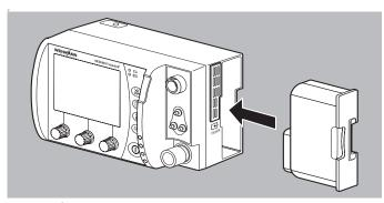
3. Slide full battery into the battery compartment until it clicks into place.
