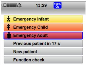
If the device was switched off for < 30 seconds (e.g., for a battery change), a countdown in the **Previous patient** field counts down 20 seconds.
