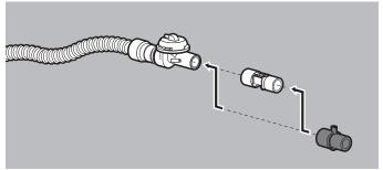
5. If available: Connect the connector with  $CO_2$  connection.
