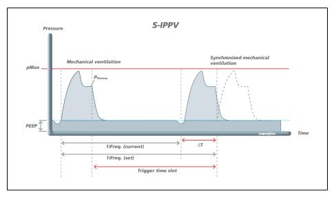
The S-IPPV mode is used for volume-controlled ventilation with a variable mandatory minute volume. Throughout the entire expiration phase, a trigger is active which enables the patient to trigger a new breath. This means the patient has the option of increasing the respiratory rate and therefore the minute volume and adapting these to his/her needs. As a rule this mode is used on patients who have inadequate spontaneous respiration.
