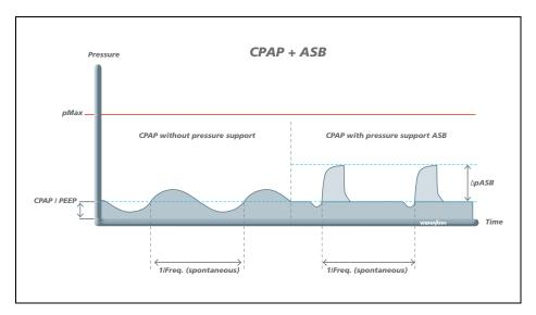
The CPAP + ASB mode can be separated into its individual elements:
