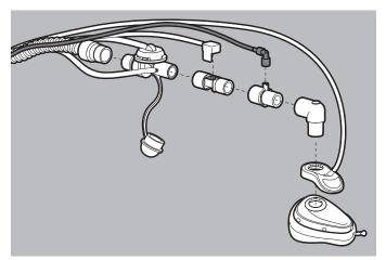
9. If available: Connect the  ${\rm CO_2}$  measuring hose to the connector with  ${\rm CO_2}$  connection.
