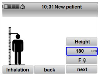
Select the height and gender: The height is given in 5 cm increments between 50 cm and 250 cm.
