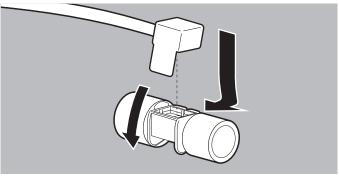
3. Hook the FlowCheck sensor connector onto the FlowCheck sensor and push down until it audibly clicks into place.
