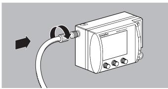
4. If necessary: Connect a low-pressure hose to the compressed gas connection of the device.
