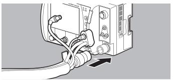
1. Connect the ventilation hose to the ventilation hose connection.
