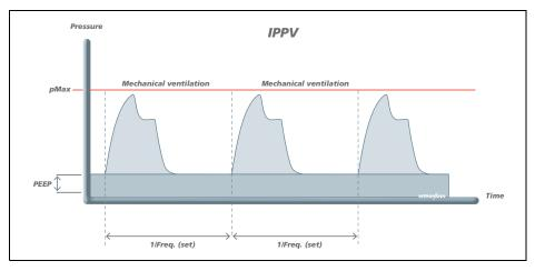
The IPPV mode is used for mandatory volume-controlled ventilation with a fixed tidal volume and fixed frequency. This mode is used on patients who have no spontaneous respiration. However, a spontaneously breathing patient can breathe deeply and freely during expiration.
