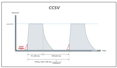
The CCSV mode is a pressure-controlled ventilation mode employed specially and exclusively for resuscitation ventilation during continuing chest compression. The ventilation mode offers you support during cardiopulmonary resuscitation (in accordance with the resuscitation guidelines) by applying a defined pressure into the lungs in time with every chest compression and switches to expiration during the chest decompression phase.
