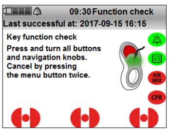
9. In the key function check, press all of the controls one after the other except for the On/Off button  $\bigcirc$ .
