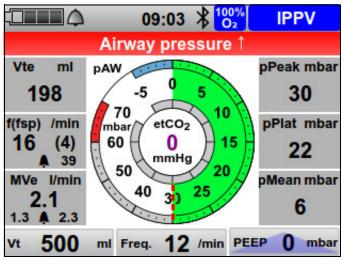
10-1 Alarm line with airway pressure alarm
