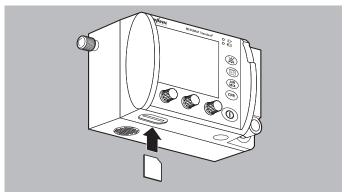
2. Slide the SD card into the SD card slot until it audibly clicks into place.
