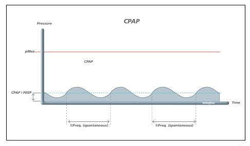
The set value CPAP/PEEP is used to increase the pressure level of respiration in order to raise the functional residual capacity (FRC) of a spontaneously breathing patient. The patient is able to breathe spontaneously without any restriction at the set pressure level. The CPAP mode is used exclusively on patients with adequate spontaneous respiration.
