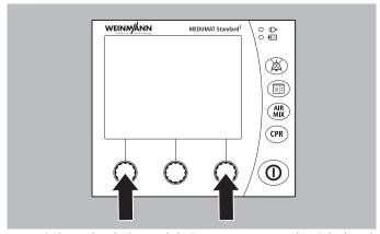
1. Switch on the device and during start-up press the right-hand and left-hand navigation knobs at the same time.
