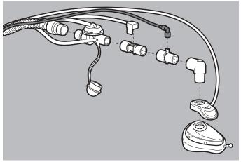
6. If available: Detach the CO<sub>2</sub> measuring hose from the connector with CO<sub>2</sub> connection.
