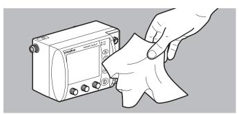
5. If the parts need to be wiped down acc. to the cleaning and disinfection plan: Wipe parts down with a clean, lint-free cloth that has been moistened with cleaning solution. When doing so, note:
