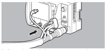
2. Connect the measuring hose system connector to the connection for the measuring hose system.
