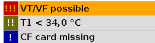
Fig. 3-16 Alarm messages in the alarm history
