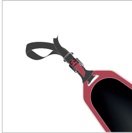
Figure 6-12 Attachment straps forming hand loops
