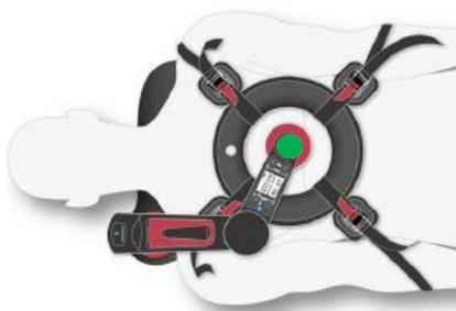
5. Close the locking lever by slapping it with the palm of your open hand and then press the green or amber LED start / stop button.
