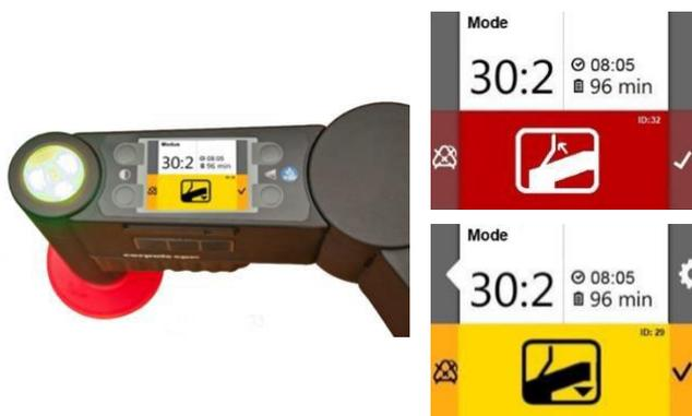
Activate and deactivate alarm suspension by pressing the soft key located beside the alarm symbol, for 3 seconds.
